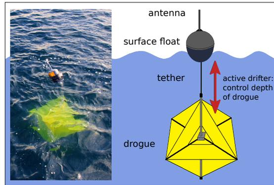
Fig. 1. Passive and active drifters. Left: A prototype of our passive drifter system, which was deployed in the Southern California Bight to measure the vectors of the ocean currents locally. Right: The schematic shows the main components and the mode of operation of a passive as well as an active drifter.
