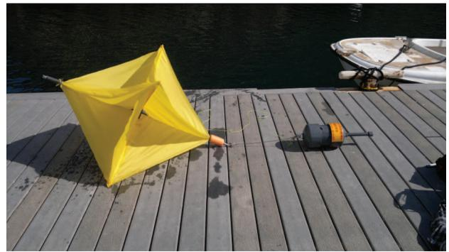
**Figure 4.** The RESL drifter. One of our three drifters when it is completely assembled. Each drifter system is composed of a drogue, a tether, and a surface float with a radio antenna.
